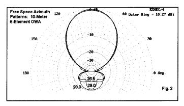
The antenna pattern itself is a model of good behavior, with no undesirable side or rear lobes. Note in Fig. 2 the change in the shape of the rearward lobe across the band, which is a normal progression for well-behaved antennas of this type.
